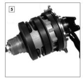
Lie the gearbox on its side and remove and dispose of the excess oil that is sitting in the hub casing.
