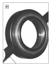
Place the new hub seal around the centering collar of the press tool. The closed side of the new hub seal faces towards the tool itself, the open side is visible.
