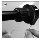
Check that the Shifter Cables run smoothly by pulling on each cable end alternatively. The Grip Rubber should rotate freely between both bed-stops <u>slightly beyond gears #1</u> and #14.
