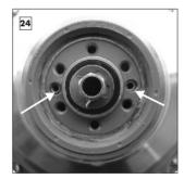
Lay the wheel on a flat surface so that the two locating peg holes (not threaded) lay at positions 3 and 9 o'clock (arrowed).
