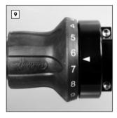
Rotate the Grip Rubber so that the gear indicator arrow falls **between** gears #6 and #7. Hold the Shifter in this position.
