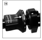
When connecting both components, slide the Grip Rubber fully over the Shifter Housing and lightly rotate until it falls into position in the Cable Pulley.
