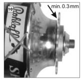
There must be a minimum of 0.3mm between the sprocket and the hub casing. If not, then remove the sprocket and push the hub seal as far back as possible. Refit the sprocket and check that the sprocket runs smoothly.
