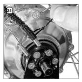
Place a new concertina tube and male bayonet connector over the cable. Tighten up the connector as with the other. Pull the shorter cable until both of the hub cables are approx. the same length. Place the two new concertina tubes over the cable guides and secure with cable ties. Make sure that the cable ties clamp the concertina tubes over the recess in each of the cable guides.
