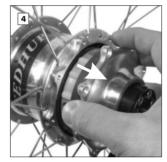
Draw the gearbox out of the hub casing. If this proves to be difficult, than gently tap the sprocket side of the gearbox with a rubber mallet to ease the process. CAREFUL! Excess oil could still leak out of the hub casing!
