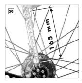
Check the rear (14) side cable is pulled out to its end stop. Measure\* this rear (14) cable and cut it at 165mm with sharp wire cutters. Place a new concertina tube carefully over the cable and place the male bayonet connector onto the end of the cable.
