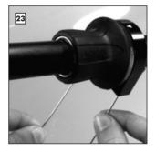
Refit the Shifter Cables into the Twist Shifter as described in the mounting instructions - Fig 6 to 11.
