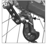
To lubricate the chain tensioner, place a drop of oil on the left and right side of the upper jockey wheel on the pivot point.
