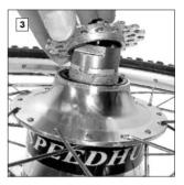
The sprocket can be removed over the sprocket tool. When only reversing the sprocket, clean the sprocket turn it over 180° and screw it back onto the cleaned and regreased thread of the driver in a clockwise direction. Tighten up the sprocket using the chain whip. If the sprocket needs to be replaced, simply screw the new sprocket tightly onto the driver.
