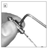
Use the 2mm allen key to secure the cable inside the bayonet connector with 0.8Nm. Secure the concertina tubes with cable ties.
