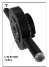
Prepare the hub seal press tool as shown in the picture.
