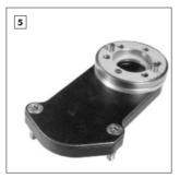
Place a new paper gasket over the locating pegs of the external transfer box, so that all holes meet up with corresponding screw holes of the axle ring. The smaller seal sits in the recess on the rear side of the axle ring.
