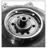
Use a cottonbud to clean and degrease (petroleum/brake cleaner) the mating surface ready for the new hub seal.
