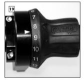
Rotate the Shifter (with fitted Cable Stoppers) until the gear indicator on the Shifter Housing is positioned **between numbers 8** and 9. Hold the Shifter in this Position.
