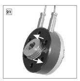
Pull the cable pulley up to the axle ring by pulling both ends of the hub cable equally. Push the cable pulley into a parallel position with the axle ring using the thumb (from outside) and index finger (from inside) whilst keeping the tension applied to both hub cable ends. The cable pulley then springs into the axle ring hole.
