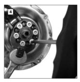
To hold the axle steady, grip the long torque arm tightly or hold the OEM or OEM2 axle plate with a 10mm wrench (see chapter "Mounting", paragraph 4.3).
