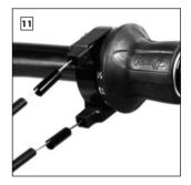
Mounting of Cable Housings with integrated liners: Thread the Cable Stoppers back over each Shifter Cable and push these firmly into the Shifter Housing facing in the correct position. Make sure to fit Ferrules between Cable Housing and Cable Stoppers.
