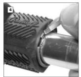
The safety ring can now be remounted. Check that the twist shifter rotates smoothly and freely. Refit new shifter cables (see chapter "Mounting", paragraph 6. "Twist shifter").
