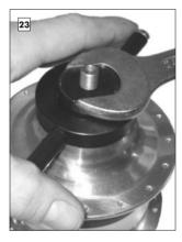
Place the sprocket tool onto the driver and se-cure it in position with the Q/R skewer or an axle nut. Set the ring over the sprocket tool and thread it clockwise as far as pos-sible over the thread of the driver whilst holding the sprocket tool still with an 24mm wrench. The new hub seal will now be pressed firmly into the correct position.
