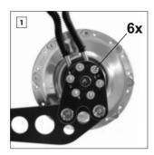
The one-piece axle ring was mounted on all internal gear mech versions until the beginning of 2003. This type of axle ring is secured to the gearbox with six axle plate screws. The cable guides of the one-piece axle ring remain fixed to the axle ring. This can be seen once the axle plate has been removed. To replace the hub cable, the axle ring complete with the cable pulley must be removed.
