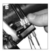
On the versions with an internal gear mech the cable adjusters can be found on the cable guide. This can be found on the left hand chain stay or attached to the left hand brake boss of the frame.
