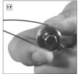
Hold both ends of the hub cable in position with thumb and index finger.
