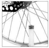
The removal procedure must start with the the rinsing and draining of the oil from within the hub (see chapter "Oil change"). The drain screw must not be reused.
