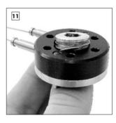
Push the cable pulley out of the axle ring from the rear side. Take care not to tilt the cable pulley for an easier removal. Remove the old hub cable and clean both the cable pulley and the axle ring. **Check cable pulley for burrs and deburr if necessary.**
