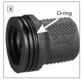
Lightly grease the twist shifter housing. The arrowed "O ring" must also be lightly greased and checked that it is sitting in the correct position before remounting.
