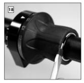
Replace the Circlip back onto the Shifter Housing. Check that the Shifter rotates freely.
