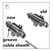
The bayonet connectors should be mounted together with the cable sheaths onto the 0.9mm hub cable. This way, damage to the cable by pincing it with the grub screws can be easily prevented.
