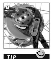
Should the axle ring not loosen by hand, use a pipe wrench to hold the axle ring tight (place cardboard between the axle ring and the pipe wrench). Rock the axle ring from side to side with the pipe wrench whilst pulling it upwards in order to loosen it from the hub.
