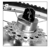
Check that the seats on the driver are clean so that the tool can be properly seated. Place the sprocket tool over the clean seats of the driver and with a quick release lever (CC) or an axle nut (TS) secure in position, so that the sprocket tool is prevented from springing out of the seats.
