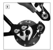
*Rohloff SPEEDHUB 500/14* versions with external gear mech: To lubricate the cable pulley bearing, remove the cable box and place a little grease on the parts arrowed in the picture above.
