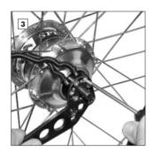
To change the hub cables, the axle plate must be first removed. To do this unscrew the six axle plate screws (M4x25 - Torx TX20).
