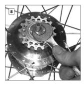
The mounting of the cable pulley must be carried out in gear #14. To do this, the axle has to be held steady with a 17mm wrench on the aluminum nut (sprocket side).
