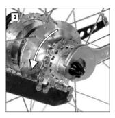
Remove the sprocket using a chain whip and the sprocket tool (see chapter "Service", paragraph 3. "Sprocket reversing/replacing").
