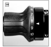
Rotate the Shifter (with fitted Cable Stoppers) until the gear indicator on the Shifter Housing is positioned **between numbers 8** and 9. Hold the Shifter in this Position.
