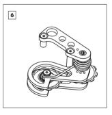
The long leg of the spring now sits against the cone washer and holds the cage back creating the tension.
