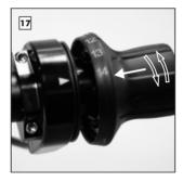
When connecting both components, slide the Grip Rubber fully over the Shifter Housing and lightly rotate until it falls into position in the Cable Pulley.
