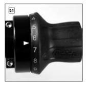
Rotate the Shifter (with fitted Cable Stoppers) until the gear indicator on the Shifter Housing is now positioned **between numbers 6 and 7.** Hold the Shifter in this Position.
