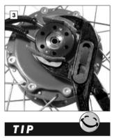
Should the axle ring not loosen by hand, use a pipe wrench to hold the axle ring tight (place cardboard between the axle ring and the pipe wrench). Rock the axle ring from side to side with the pipe wrench, whilst pulling it upwards in order to loosen it from the hub.
