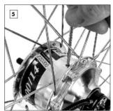
Fit a new oil drain screw and tighten correctly (Allen Key SW3, tightening torque 0.5Nm). As long as the thread sealant is not worn, then the old oil drain screw may be used repeatedly.
