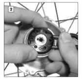
Lie the wheel on a flat surface with the axle ring facing up and the cable guides facing to the right. Rock the axle ring from side to side whilst pulling it upwards in order to loosen it from the hub.
