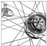
Check the function of the axle ring by gripping one end of the hub cable with pliers and pulling this out to the end stop. Repeat this process with the other end of the hub cable. At the end stops, both ends of the hub cables should protude from the cables guides by the same amount.
