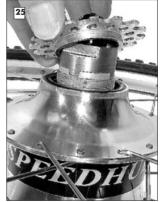
Replace the new/rotated sprocket (with undamaged seal surfaces) as shown in the Owners Manual.
