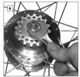
The mounting of the cable pulley must be carried out in gear #14. To do this, the axle has to be held steady with a 17mm wrench on the locking nut on the sprocket side.
