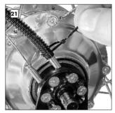
Place a new concertina tube and male bayonet connector over the cable. Tighten up the connector as with the other. Pull the shorter cable until both of the hub cables are approx. the same length. Place the two new concertina tubes over the cable guides and secure them with cable ties. Make sure that the cable ties clamp the concertina tubes over the recess in each of the cable guides.
