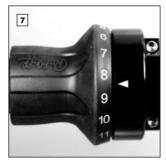
Rotate the Grip Rubber so that the gear indicator arrow falls **between** gears #8 and #9. Hold the Shifter in this position.
