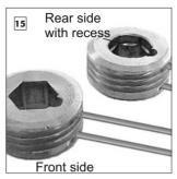
Pay attention to which side of the cable pulley is the mounting side. The back/mounting side has a recess before its hexagonal hole. The front side is without this recess.
