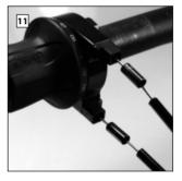
Mounting of Cable Housings with integrated liners: Thread the Cable Stoppers back over each Shifter Cable and push these firmly into the Shifter Housing facing in the correct position. Make sure to fit Ferrules between Cable Housing and Cable Stoppers.
