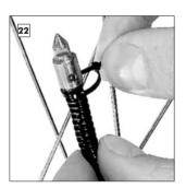
The top ends of the concertina tubes must be placed over the ends of the male bayonet connectors and secured with cable ties. Make sure that the cable ties clamp the concertina tubes over the recesses.
