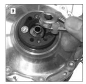
Lie the wheel on a flat surface with the axle ring facing up and the cable guides facing to the right. Pull the cable guides with the nylon cylinders and the cable pulley upwards and out of the axle ring.
