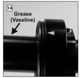
Before fitting the replacement Grip Rubber, check that the O-ring is seated correctly on the Cable Pulley.
