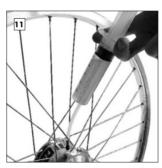
Refill the *Rohloff SPEEDHUB* 500/14 with 25ml of *Rohloff SPEEDHUB OIL* (see chapter "Service", paragraph 1. "Oil change") and refit a new drain screw (3mm allen key, tightening torque: 0.5Nm/4in.lbs.).
