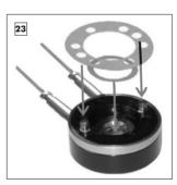
Place a new paper gasket over the locating pegs of the axle ring so that all holes meet up with the corresponding screw holes of the axle ring. The smaller gasket sits in the recess on the rear side of the axle ring.
