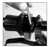
Both Clamp Screws (M3x12 - Torx TX20) should be lightly fitted so that the gap between both clamp elements is identical.
