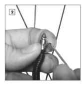
Unscrew both bayonet male connectors from the hub cables (M4x4 - 2mm allen key) and remove the concertina tubes.
