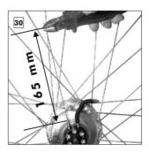
Push the cable up into the male bayonet connector as far as it will go and tighten both 4mm headless screws (2mm allen key, tightening torque: 1.5Nm/12"lbs.). Pull the front (1) side cable with pliers through the 13 clicks of the gearbox until the endstop (gear #1). Measure\* this front (1) cable and cut it at 165mm with sharp wire cutters.
