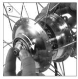
The gearbox only sits properly once the joints sit in their correct positions against the hub casing. To ease the process, rotate the driver in clockwise direction whilst pushing the two parts together.
