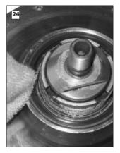
Remove the ring and the sprocket tool.
