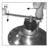
Lay a 10mm wrench flat over the sprocket tool with the open end hooked under the wooden grip of the removal tool. Secure the removal tool by pushing it against the sprocket tool. Force the wrench down onto the sprocket tool in order to lever the removal tool with the old hub seal upwards and out of the hub shell. Remove the insert.
