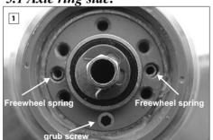
Lie the wheel on a flat surface with the sprocket side facing down. Remove the axle plate and the corresponding gear mech - a brake disc may have to be removed for this procedure.
