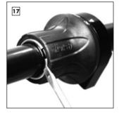
Replace the Circlip back onto the Shifter Housing. Check that the Shifter rotates freely.
