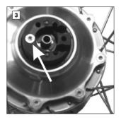
Remove the axle ring screw (M4x20 - Torx TX20) and rock the axle ring from side to side, whilst pulling it upwards in order to loosen it from the hub.
