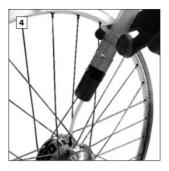
Draw 25ml SPEEDHUB OIL into the syringe and insert this into the hub. Draw out approx. 25ml of air to keep the pressure correct inside and therefore, avoid oil seeping back out, when removing the filling tube.
