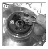
The axle ring remains attached to the axle by one more countersunk head bolt underneath the axle plate. Lie the wheel on a worktop with the axle ring facing upwards. Remove the two cable guides with the nylon cylinders and the cable pulley by rocking the cable guides from side to side until they are released from their seats within the axle ring.
