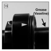
Before fitting the replacement Grip Rubber, check that the O-ring is seated correctly on the Cable Pulley.
