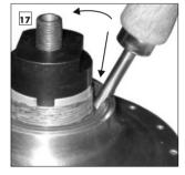
Remove the old hub seal from the hub shell. To do this place the sprocket tool onto the driver and hook the removal tool under the old hub seal. Lever the removal tool into the upright position as shown in the picture.
