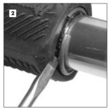
With a flat screwdriver, remove the safety ring. The rubber grip can now be removed. Clean the twist shifter housing.
